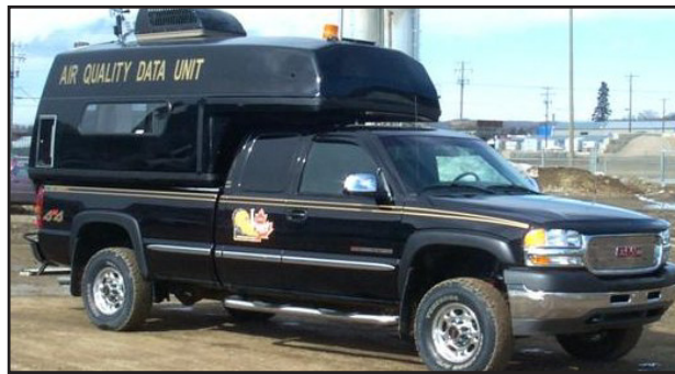
▲ KMS also offers the DWM technology, which provides more accurate analysis of SO 2 and H 2 S concentrations, but isn't as portable as the C-R units. Shown here is one of nine units that is available through the KMS division.
