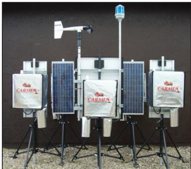
▲ The solar-powered, portable CARMEN-REACTOR sensors monitor ambient air quality and provide remote, real-time data to a secure Internet site.
